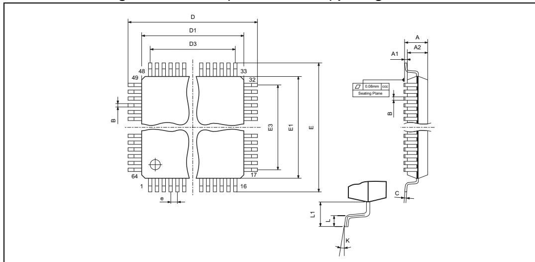
Table 19. TQFP64 (10 mm x 10 mm) mechanical data
