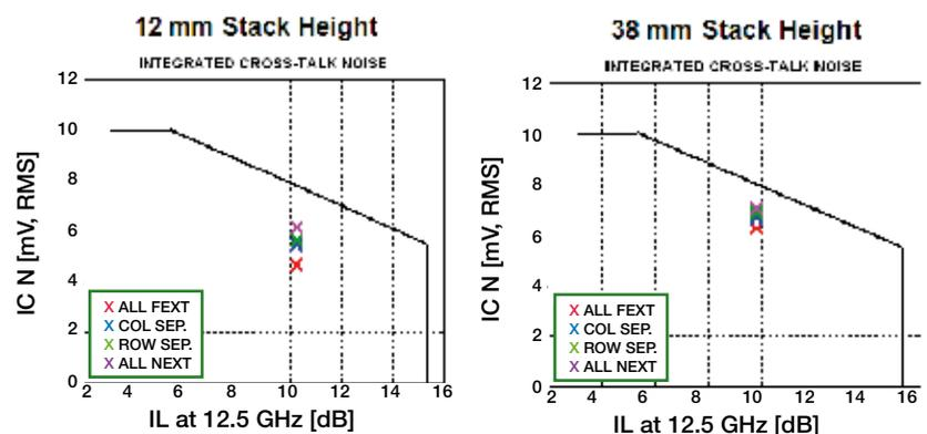
ICN (Integrated Cross-Talk Noise) is shown for links simulated with 150 mm of traces -> Footprint -> TwinMezz 12 / 38mm connector -> Footprint -> 150 mm of traces. (wiring patterns below)
