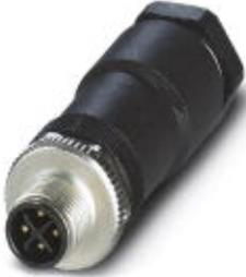
Connector, 4-position, Plug straight M12, S-coded, Screw connection, Knurl material: Zinc die-cast, nickel-plated, Cable gland Pg11, External cable diameter 8 mm ... 10 mm
