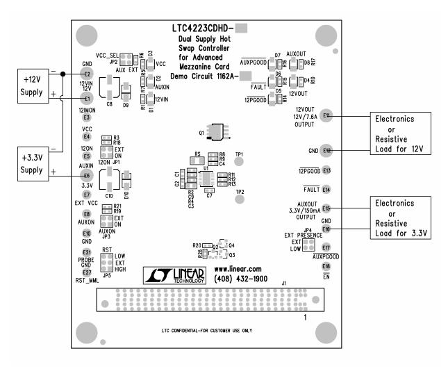
Figure 1. Measurement Equipment Setup
