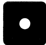
Q- Square Bezel Snap-on (FM) Cutout Standard- 1.437in. Miniature- 1.250in.
