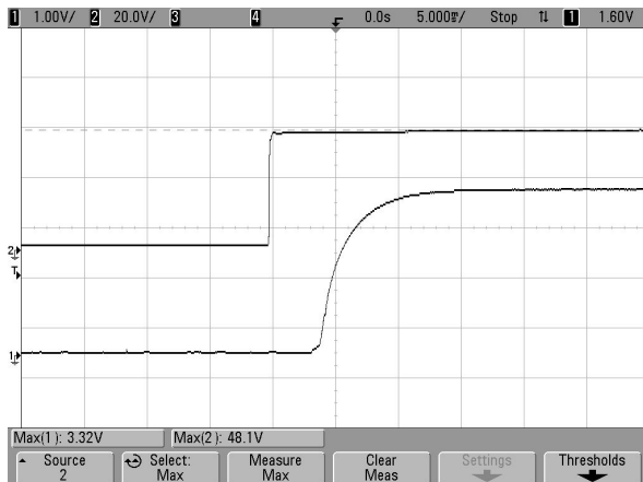
Figure 3 Typical start-up from power on
