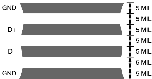
Figure 22. Typical Arrangement of Signal Tracks
