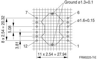
Hole arrangement View in mounting direction (Note half pitch!)
