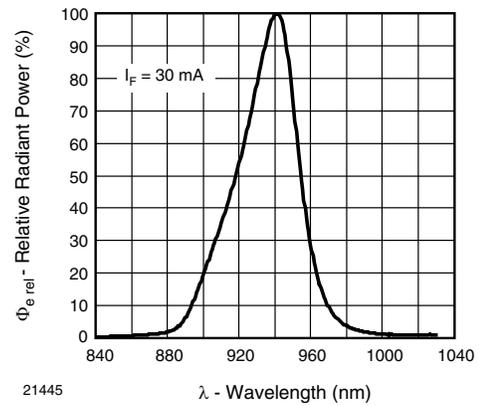
Fig. 7 - Relative Radiant Power vs. Wavelength
