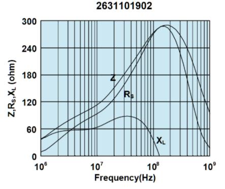
Impedance, reactance, and resistance vs. frequency.
