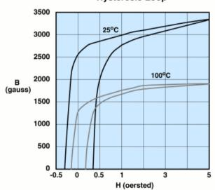
Measured on a 17/10/6mm toroid at 10kHz.
