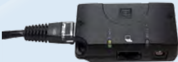
Power LED illuminates when connected to compliant IEEE802.3af load.
