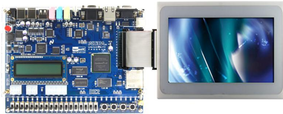
Figure 5-8 Hardware Setup with DE2-115
