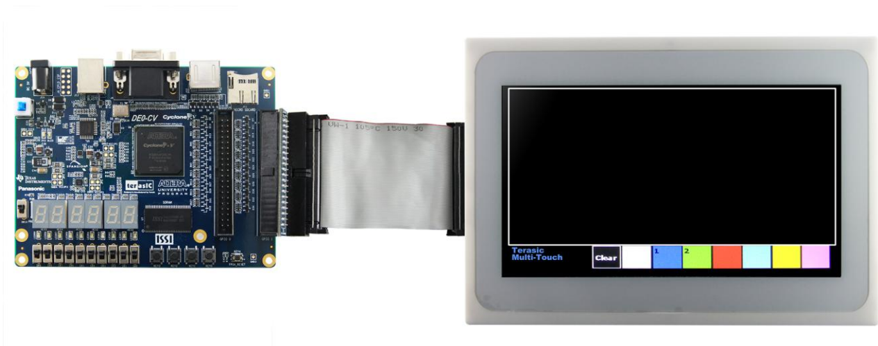
Figure 5-7 Hardware Setup with DE0-CV
