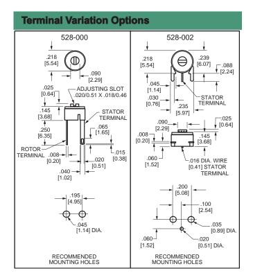
For dimensions  $\geq$  .126"/3.20mm, tolerance is ±.015/0.38 For dimensions  $\leq$  .125"/3.18mm, tolerance is ±.005/0.13
