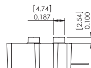
C- Two Ports Cut 0.100" Configuration
