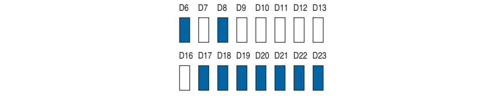
Figure 4-14. Condition of LEDs for Transmitting 3G-SDI Level B Video Standard
