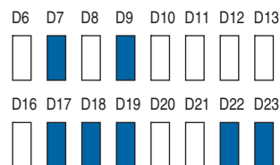
Figure 4-12. Condition of LEDs for Transmitting HDI-SDI Video Standard
