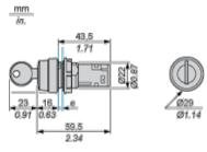
e Support panel thickness: 1 to 6 mm/0.4 to 0.24 in. (metal), 2 to 6 mm/0.8 to 0.24 in. (plastic).
