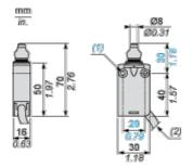
(1) 2 fixing holes Ø 4.2 mm, counterbored Ø 8 mm by 4 mm deep.
