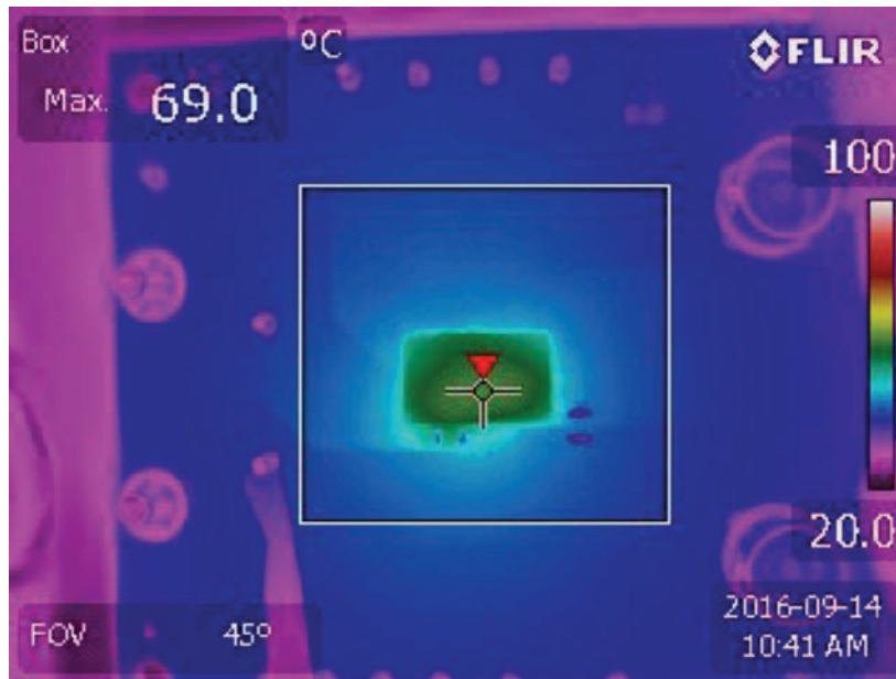
Figure 4. Thermal Image of LTM4647, V_{IN} = 12V , V_{OUT} = 1.0V , I_{LOAD} = 30A , T_A = 23.0^{\circ}C , No Forced Air Flow
