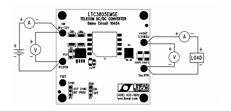
Figure 1. Proper Measurement Equipment Setup
