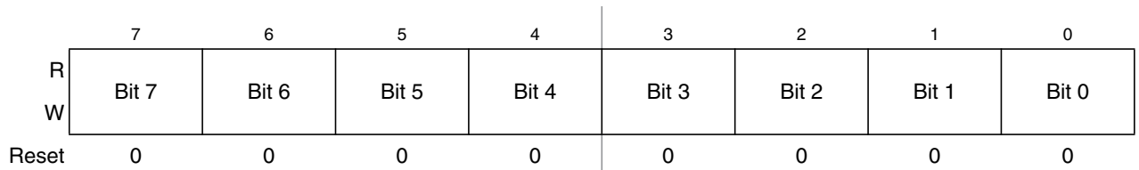
Figure 12-23. Timer Input Capture/Output Compare Register x Low (TCxL)
