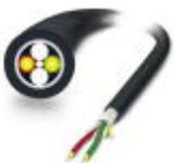
Highly rugged HCS round cable (IP20 heads only) for assembly and for outdoor installation with integrated moisture barrier as well as rodent-proof scrim. Individual elements made from highly flexible FRNC material. The wire is ozone and UV resistant with a very rugged polyethylene outer sheath.
