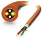
rugged HCS installation cable for inner areas with highly tear-proof aramid strain-relief elements. Individual elements made from highly flexible FRNC material. The cable is halogen-free, ozone and UV resistant and has a rugged polyurethane (PUR) outer sheath.
