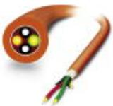
rugged HCS installation cable (IP20 heads only) for inner areas with highly tear-proof aramid strain-relief elements. Individual elements made from highly flexible FRNC material. The cable is halogen-free, ozone and UV resistant and has a rugged polyurethane (PUR) outer sheath.
