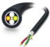
Highly rugged HCS round cable for assembly and for outdoor installation with integrated moisture barrier as well as rodent-proof scrim. Individual elements made from highly flexible FRNC material. The wire is ozone and UV resistant with a very rugged polyethylene outer sheath.
