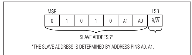
Figure 2. DS3501 Slave Address Byte
