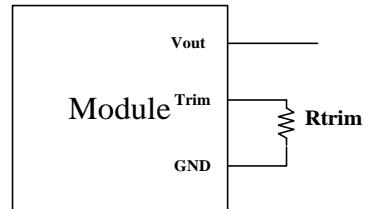
Equation for calculating the trim voltage (in V) given the desired adjusted voltage ( $V_{adj}$ ) is shown below. The Trim Up voltage should be connected between the Trim pin and Ground.
