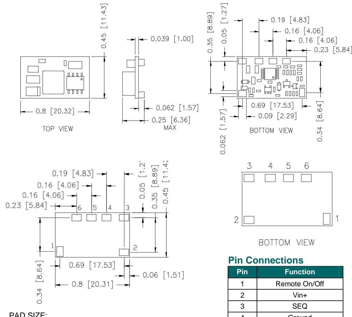
**Note:** These parts are not however compatible with the higher temperatures associated with lead free solder processes and must be soldered using a reflow profile with a peak temperature of no more than 245 °C.
