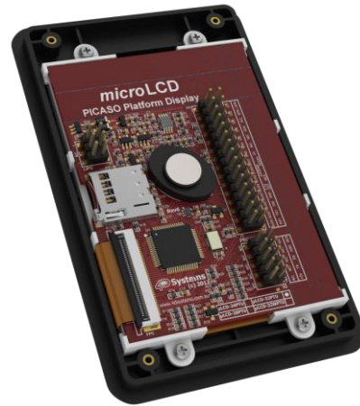
uLCD-32PTU Mounted in 3.2" Bezel - Back
