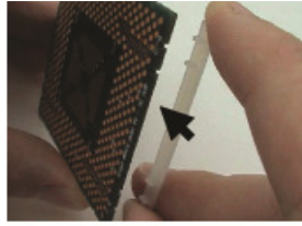
Figure 1 – Schmart mechanical bridge being connected to a SchmartBOARD™.
