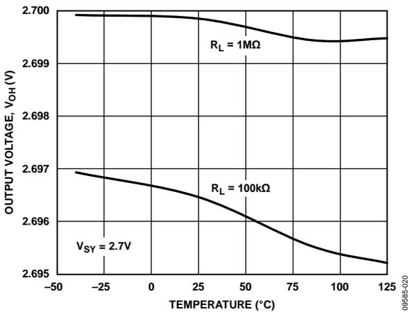
Figure 17. Output Voltage ( $V_{OH}$ ) vs. Temperature
