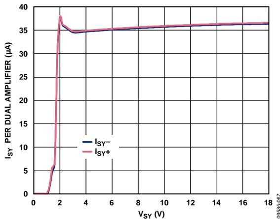
Figure 66. Supply Current vs. Supply Voltage (Voltage Follower)
