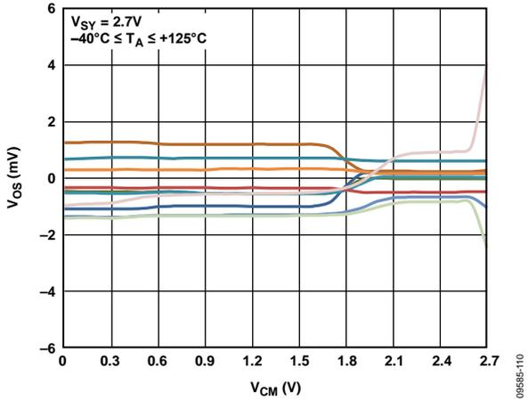
Figure 9. Input Offset Voltage vs. Common-Mode Voltage
