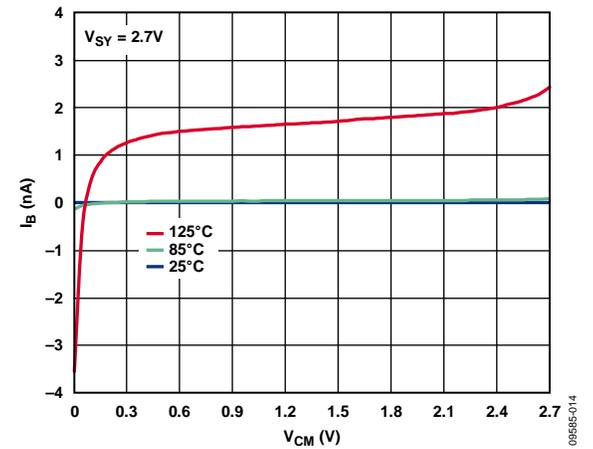
Figure 11. Input Bias Current vs. Common-Mode Voltage
