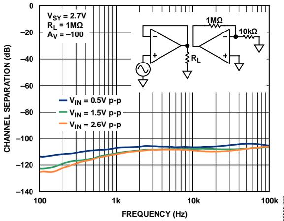
Figure 58. Channel Separation vs. Frequency
