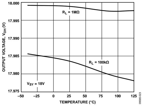
Figure 20. Output Voltage ( $V_{OH}$ ) vs. Temperature
