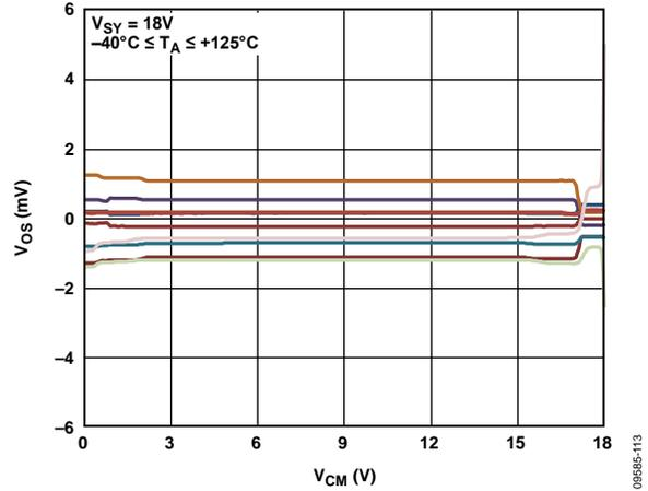
Figure 12. Input Offset Voltage vs. Common-Mode Voltage
