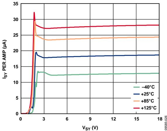
Figure 23. Supply Current per Amplifier vs. Supply Voltage
