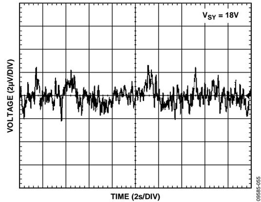
Figure 55. 0.1 Hz to 10 Hz Noise
