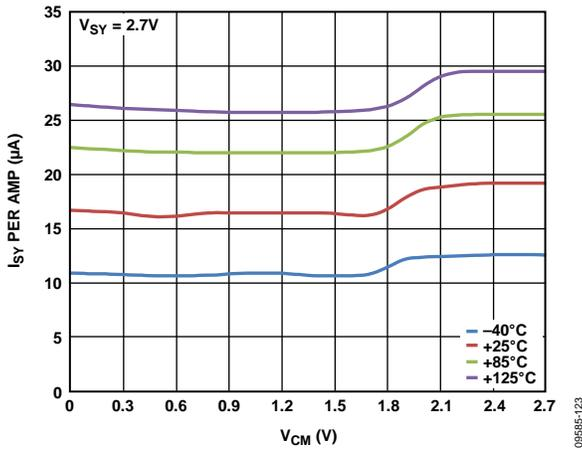
Figure 22. Supply Current per Amplifier vs. Common-Mode Voltage
