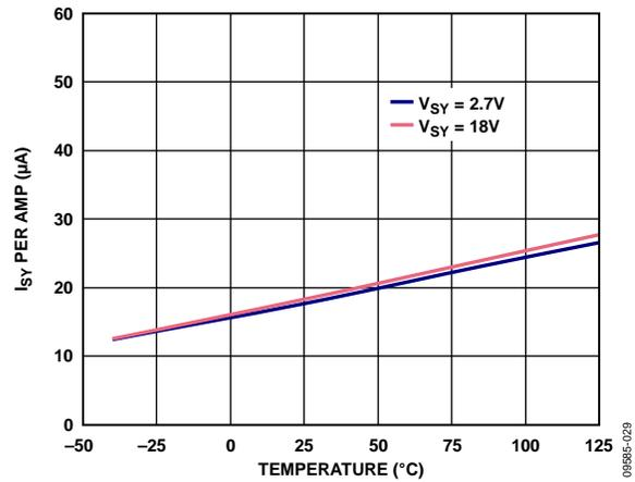
Figure 26. Supply Current per Amplifier vs. Temperature
