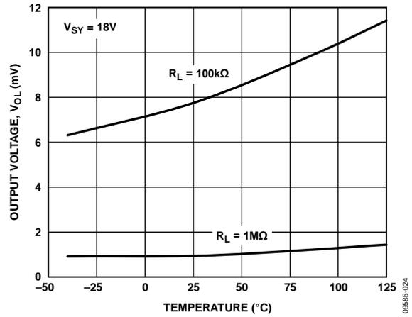
Figure 24. Output Voltage ( $V_{O}$ ) vs. Temperature
