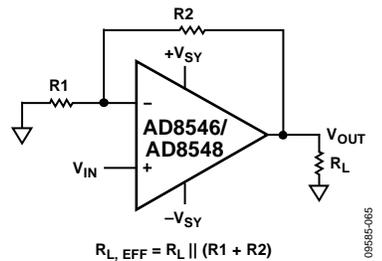
Figure 64. Noninverting Op Amp Configuration
