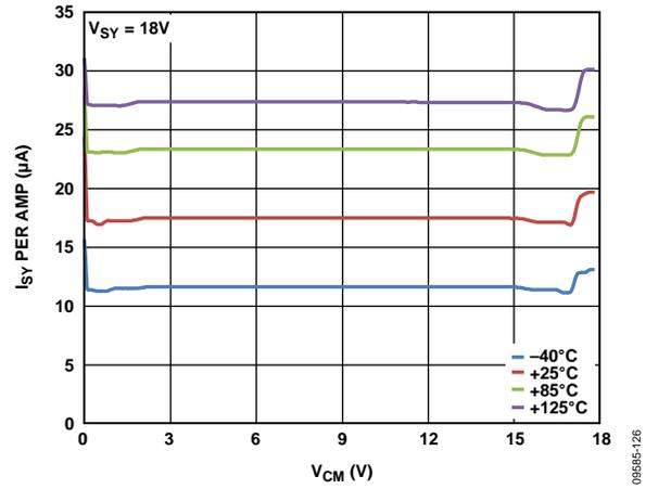
Figure 25. Supply Current per Amplifier vs. Common-Mode Voltage
