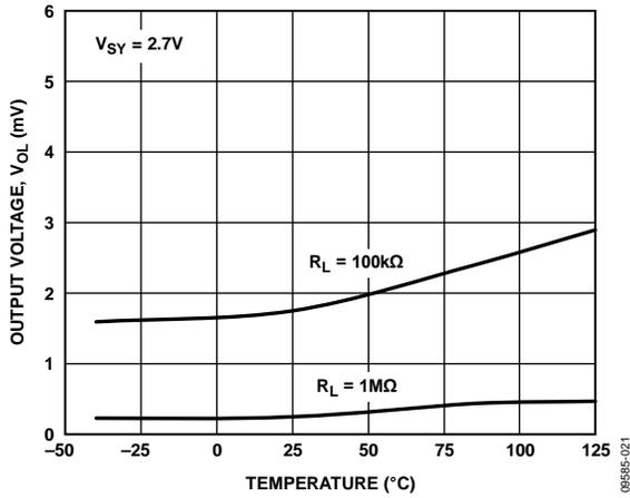
Figure 21. Output Voltage ( $V_{O}$ ) vs. Temperature
