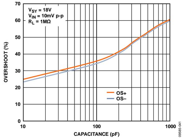
Figure 38. Small Signal Overshoot vs. Load Capacitance
