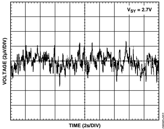
Figure 52. 0.1 Hz to 10 Hz Noise
