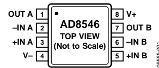
Figure 1. AD8546 (8-Lead MSOP)
