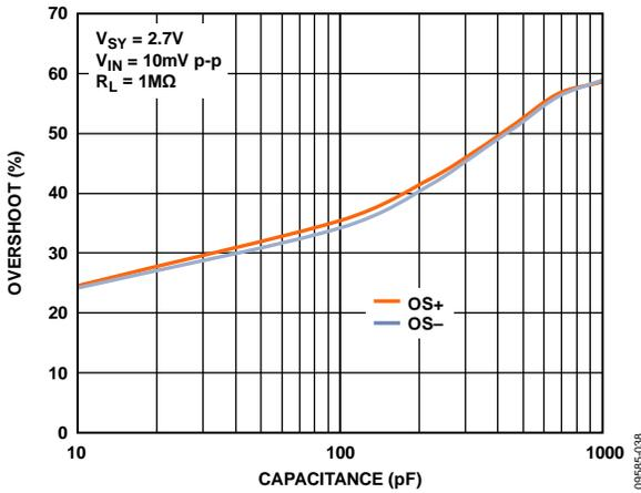
Figure 35. Small Signal Overshoot vs. Load Capacitance
