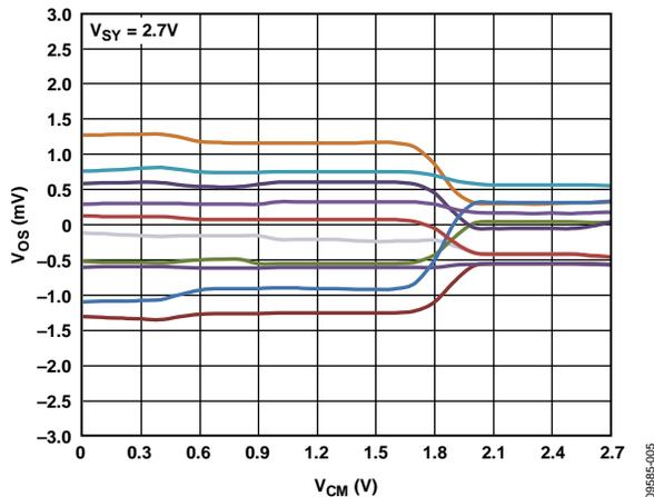
Figure 5. Input Offset Voltage vs. Common-Mode Voltage
