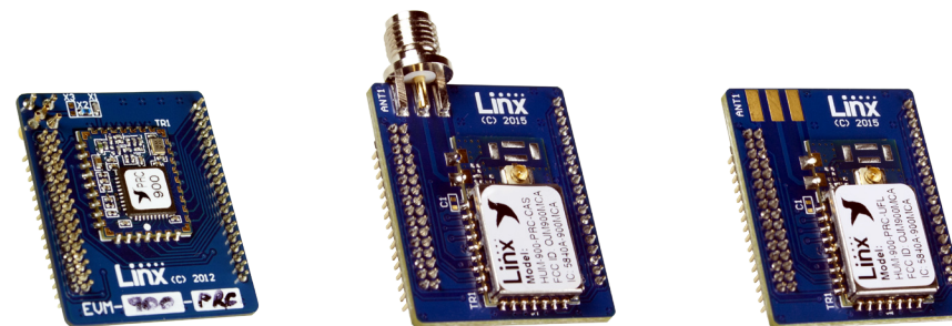
Figure 1: HumPRC™ Series Evaluation Modules; from left: EVM-***-PRC, EVM-***-PRC-CAS, EVM-***-PRC-UFL
