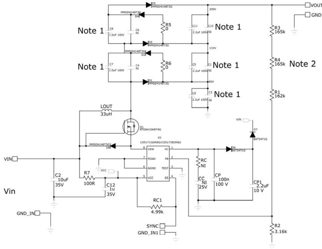
Note 1: The designer should choose either an electrolytic capacitor or a ceramic capacitor both are not required
