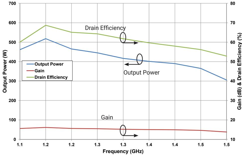
**Figure 4. - CGHV14500 Typical CW RF Results**
