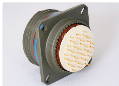
D38999 Connector with PC Tail Coax Contacts, Sealing Plugs in unused contact cavities and PC Tail Alignment Disc
