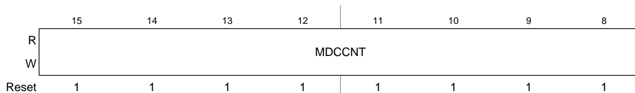
Figure 21-6. Modulus Down-Counter Count Register High (MDCCNT)
