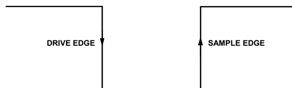
Figure 78. SPI Mode 0 SCLK Edges
