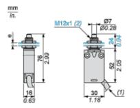
(1) External diameter of cable 7.5 mm.
