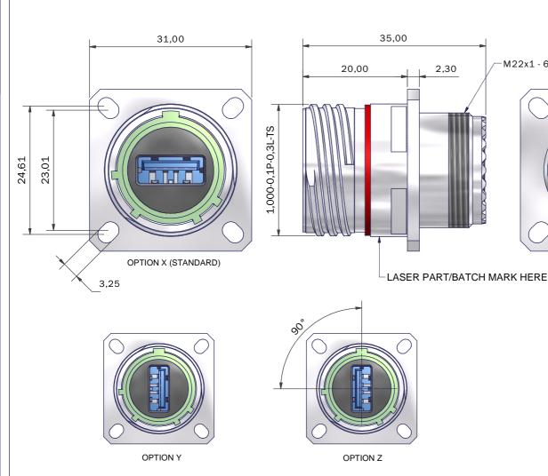
GENERALLY TO THE REQUIREMENTS OF MIL-DTL-38999 MATES WITH AMPHENOL USBFTV AND USB3FTV
