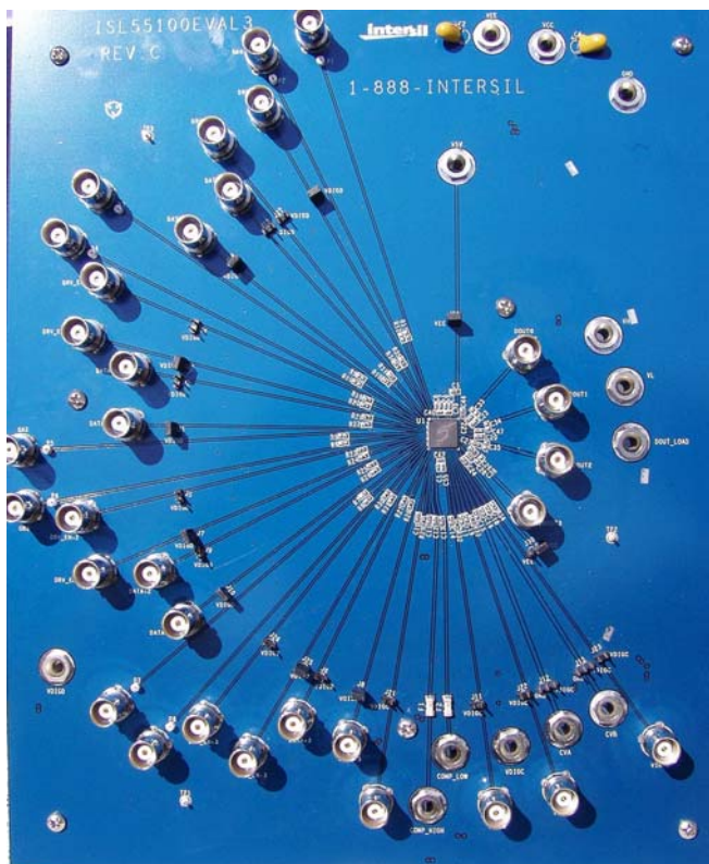
FIGURE 4. ISL55100A/BEVAL3/3Z EVALUATION BOARD
