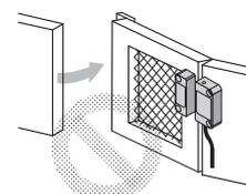
12. Where two or more Switches are mounted side-by-side, they must be no closer than 25 mm.
