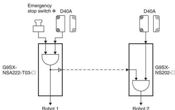
\* A manual reset is required when an emergency stop is used.
