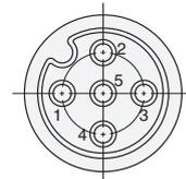
**Sockets and Plugs on Cable Ends (5-pole Connectors)**
