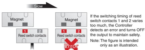
**Stable Detection with the D40A's New System**
