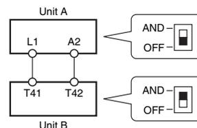
**Note:** A setting error will occur and Unit B will lock out if the logical AND setting switch on the Unit B is set to OFF.
