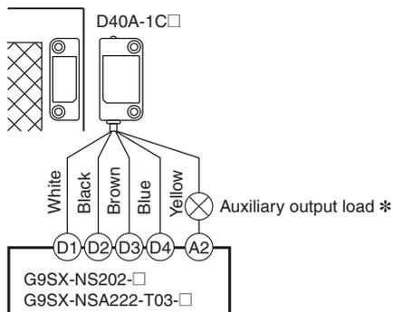
\* The auxiliary output load current must be 10 mA max.
