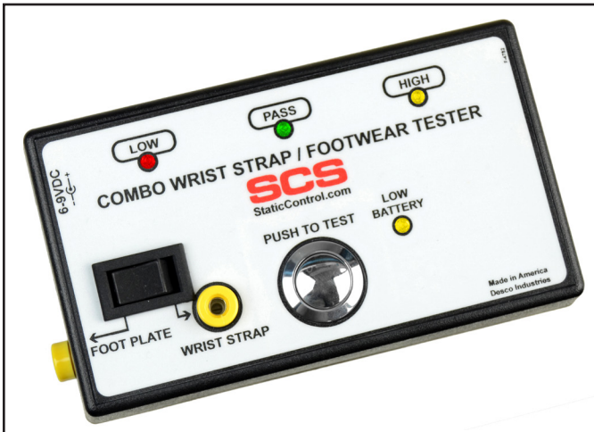
Figure 1. SCS 770030 Combo Tester
