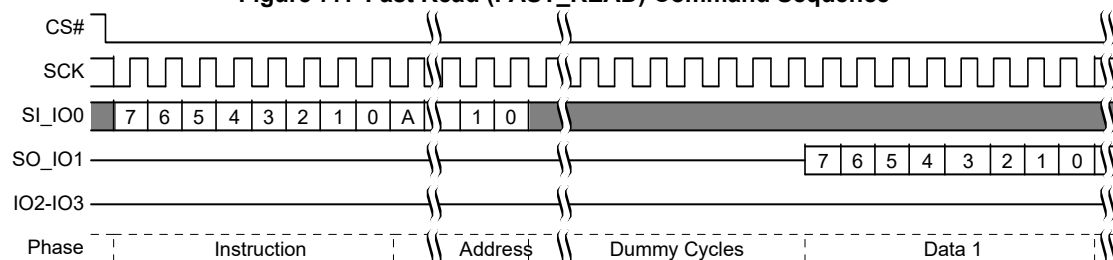
Figure 77. Fast Read (FAST_READ) Command Sequence
