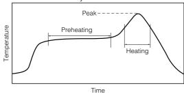
For soldering (Example: Sn/Pb)
