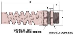
Material Nylon 6/6 w/Buna N or TPE Sealing Gland Certifications (UL) Listed under Underwriters' Laboratories File E51579 Recognized under the Component Program of Underwriters' Laboratories File E51579 Certified by Canadian Standard Association File 93876C Approved for NEMA 4, 4X, 6 and 6P Applications
