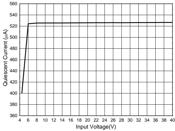
Quiescent Current vs. Input Voltage
