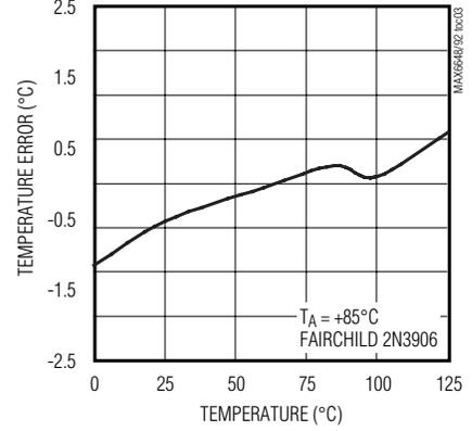
**REMOTE TEMPERATURE ERROR vs. 45nm REMOTE DIODE TEMPERATURE**
