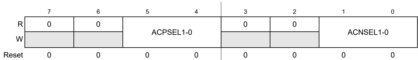
Figure 3-3. ACMP Control Register (ACMPC1)
