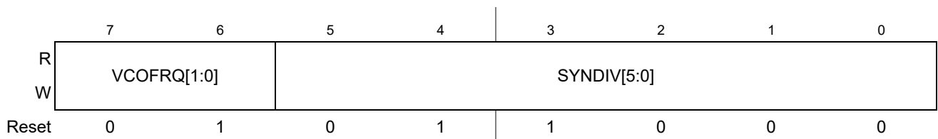
Figure 9-7. S12CPMU_UHV Synthesizer Register (CPMUSYNR)
