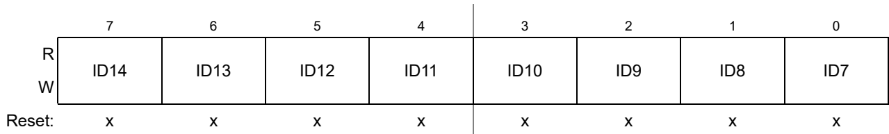
Figure 13-27. Identifier Register 2 (IDR2) — Extended Identifier Mapping
