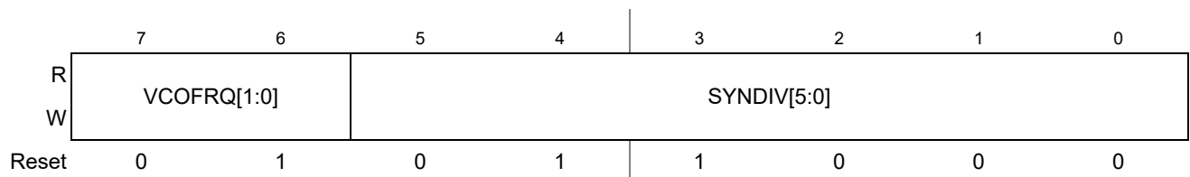
Figure 9-7. S12CPMU_UHV Synthesizer Register (CPMUSYNR)
