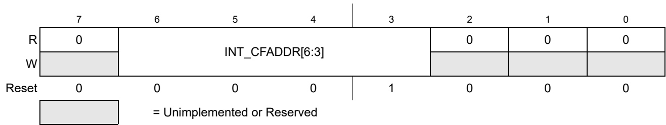
Figure 6-4. Interrupt Configuration Address Register (INT_CFADDR)
