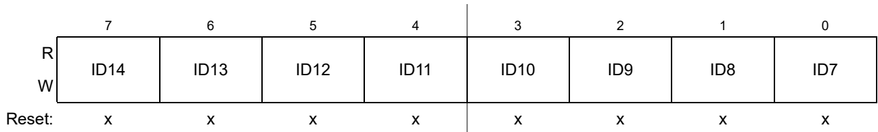
Figure 13-27. Identifier Register 2 (IDR2) — Extended Identifier Mapping
