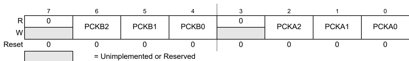
Figure 17-6. PWM Prescale Clock Select Register (PWMPRCLK)
