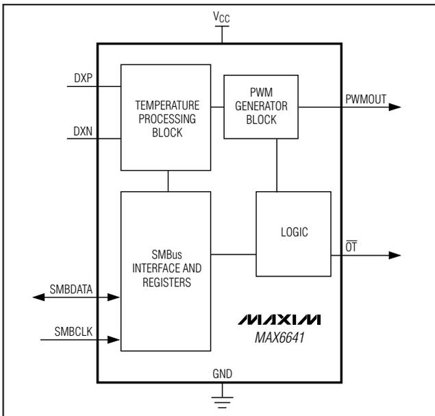
Figure 4. Block Diagram
